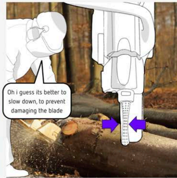
The handle transforms to a slimmer shape with the intention of discouraging the user from applying more force by providing less assistance on the handle.
