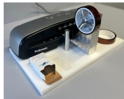
Figure 13. Homebuilt laminator for semi-automatic donor slide fabrication, for coating glass slides with self-adhesive polyimide tape.
