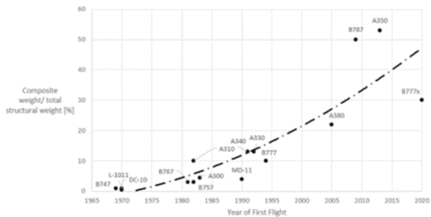
Figure 1: Share of composite material used in wide-body aircraft, 1965 – 2020. [15]
