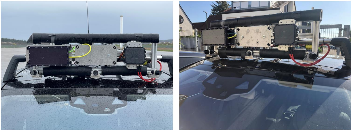
AI-SEE Prototyp 2 (uLRR) mounted on a vehicles's roof rack together with Gen5 Premium (FR5CU)
