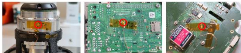
Figure 1 - Sensor positions (TS-AC-ring, TS-CB-top, TS-CB-btm)
