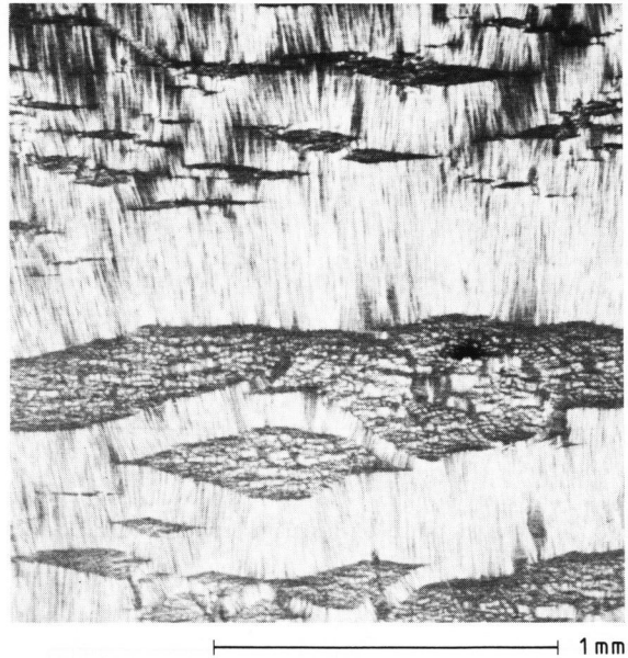
Figure 1. Partially crystallized ZBLAN preform surface of neck-down region.
