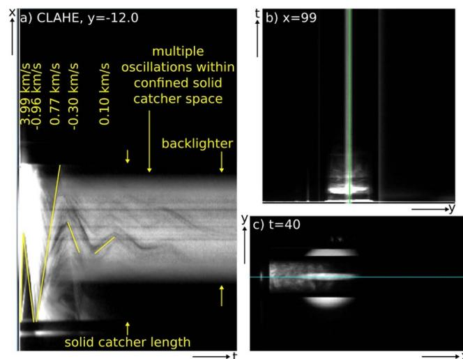
**Figure 18.** The Fiji plugin volume viewer [96] was used to obtain 3D-rendered high-speed video frames of sample 17 081, PS, Cu plate, 83.2 J, 500 kfps with the third dimension being time to deduce ejection velocities of plasma cloud features within a solid-state catcher over the course of time. The green (b) and blue line (c) show the slice positions of sub-image (a).
