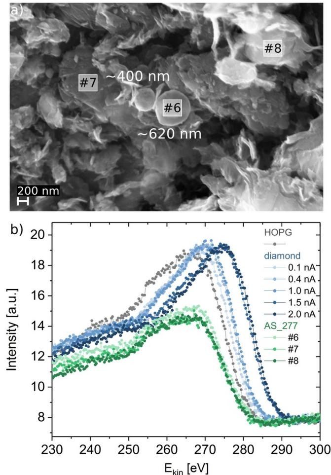
**Figure 10.** Auger electron spectroscopy (AES) analysis of sample 277, rigid graphite (RG), Ti catcher plate, 27 J. (a) SEM image displaying the AES measurement locations. Reproduced from [33]. [CC BY 4.0](#). (b) Comparison of sample spectra with recorded reference data of highly oriented pyrolytic graphite (HOPG) and diamond.
