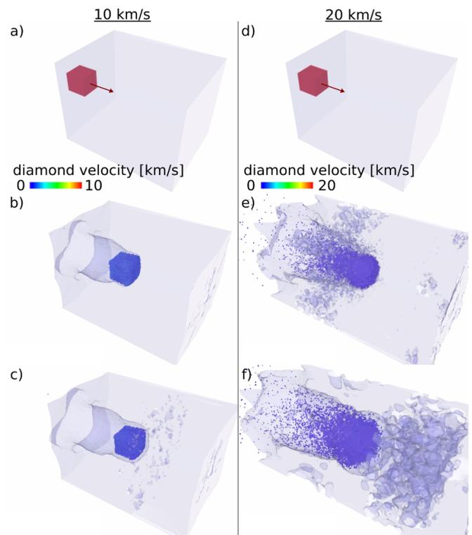
**Figure 7.** MD simulations modelling the impact of a  $\sim 6$  nm diamond cube impacting at 10  $\text{km s}^{-1}$  (a)–(c) and 20  $\text{km s}^{-1}$  (d)–(f) into a 40 nm long block of aluminium consisting of  $\sim 10^6$  atoms. Reproduced from [33]. [CC BY 4.0](#).
