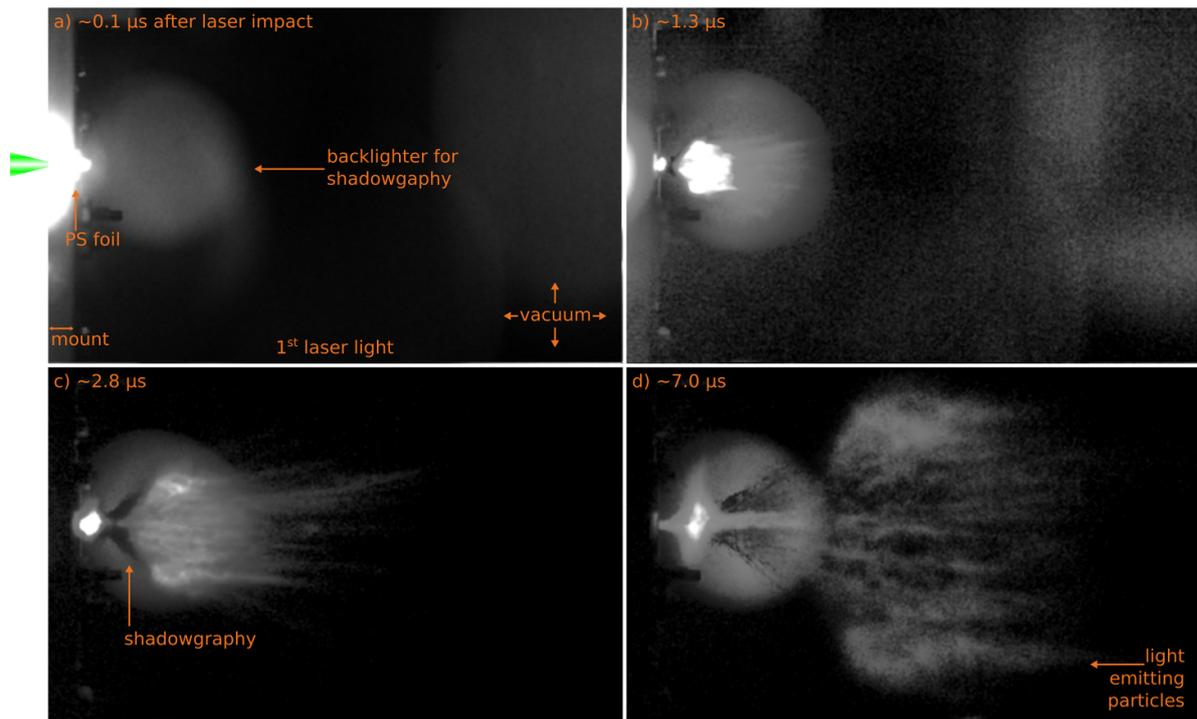
17184, PS, Cu plate, 60.4 J, 2 MHz, 500 ns/frame, field of view 52 x 32.5 mm<sup>2</sup>
