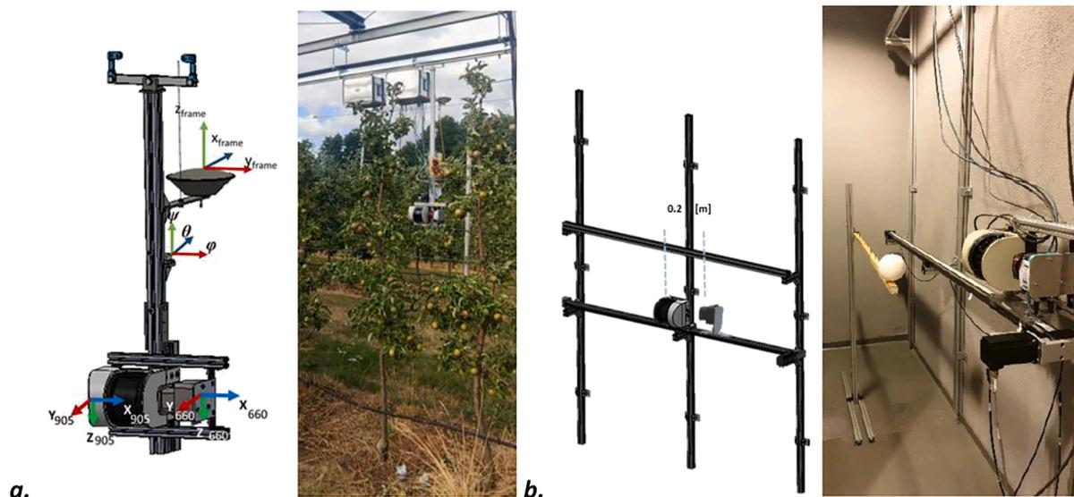
Fig. 1. Sensors mounted on a. chain conveyor to measure entire trees in the experimental orchard, and b. tooth-belt conveyor to measure individual fruit in dark room conditions.
