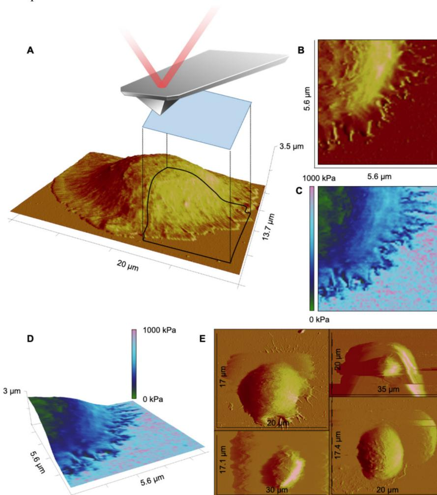
**Figure 2. AFM-based elasticity mapping (PeakForce QNM) and data analysis.**
